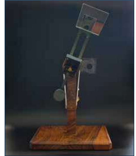
Fig. 4 The iconoscopic setup is supposed to annihilate all spatial perceptions by placing the mirror directly on top of the sighting hole for the left eye's image. Hence all parallax shifts should be reduced to zero and our brain could not make any spatial interpretations whatsoever! Credits © 2024 Andreas Junk, reconstruction of the Padua polystereoscope at the Europa-Universität Flensburg.
