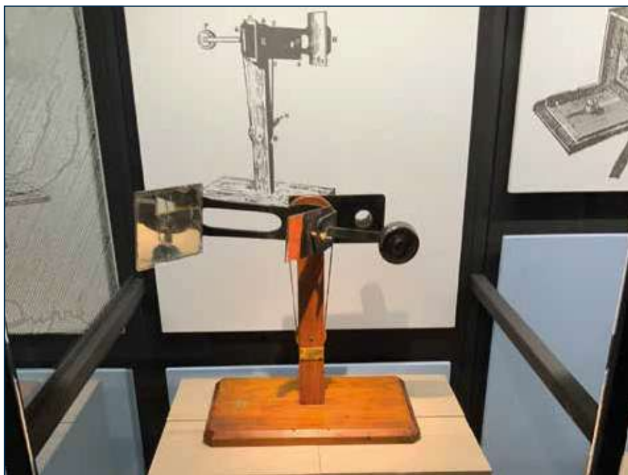
Fig. 1 The Polystereoscope on the model of Augusto Righi in the configuration for telestereoscopic observation, currently on display at the Museo Giovanni Poleni in Padua. The instrument's image in the background is taken from a summarising short paper, published by Righi in 1893. 6 Credits © 2024 Andreas Junk, Europa-Universität Flensburg.
