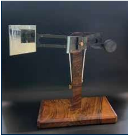
Fig. 2 The Setup, where the big mirror of the mirror arm is in a position to the right of the right eye is called telestereoscopic. The perception of spatial effects is enhanced compared to observations with the naked eye. Credits © 2024 Andreas Junk, reconstruction of the Padua polystereoscope at the Europa-Universität Flensburg.
