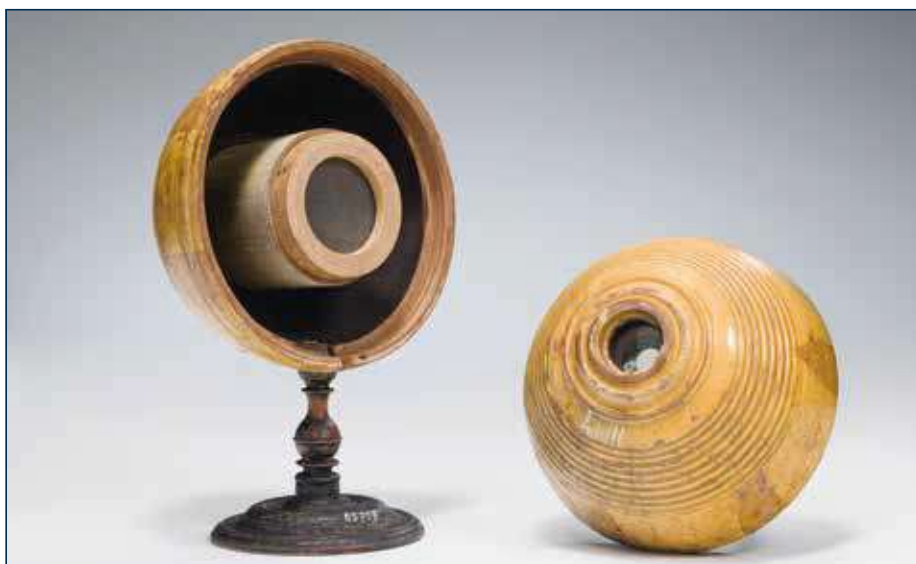
Fig. 4 Functional model of the human eye, opened in this picture. Clearly visible are the lens and the blue iris around the pinhole in the front section on the right, and the frosted glass pane standing in for the retina on the left. © Copyright: Munich, Bayerisches Nationalmuseum. Foto: Bastian Krack.
