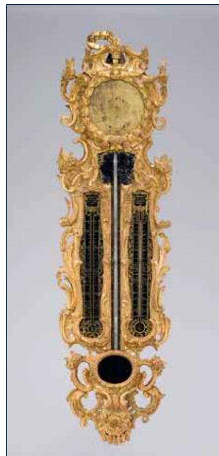
Fig. 1 Barometer-thermometer from the Würzburg Residence. In the centre the barometer; to the left the thermometer with the Réaumur scale and to the right the thermometer with the Fahrenheit scale. © Copyright: Munich, Bayerisches Nationalmuseum. Foto: Bastian Krack.
