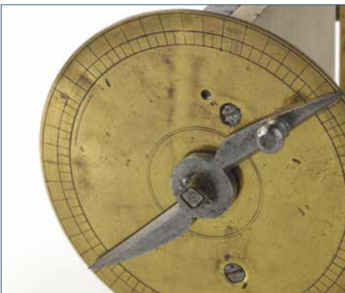
Fig.4 (a) The large dial from the same micrometer and (b) the top view of the small dial which is also shown quite clearly in Fig. 1.
