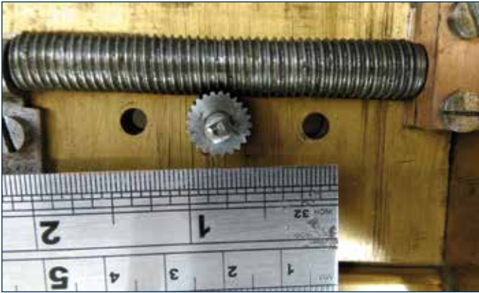
Fig. 3 (a) and (b) Two views of the lead screw from micrometer, inv. no. 1876-1370, which also clearly shows the small gear wheel which rotates the small dial.
