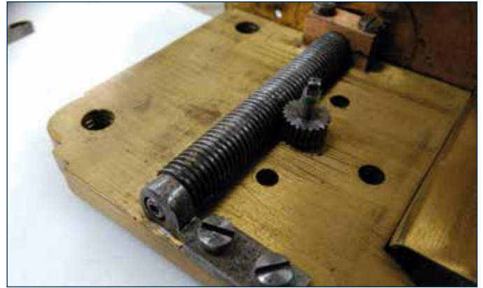
Fig. 3 (a) and (b) Two views of the lead screw from micrometer, inv. no. 1876-1370, which also clearly shows the small gear wheel which rotates the small dial.
