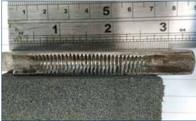
Fig. 5 The bottom of the micrometer's moveable anvil, showing the interface with the leadscrew beneath. As the leadscrew rotates, it moves the anvil along the axis of rotation. Science Museum inv. no. 1876-1370.
