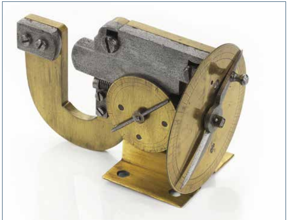
Fig.1 The alleged Watt micrometer. A workpiece is placed between the two iron anvils at top left, and the longer of the two is brought into contact by advancing it using a leadscrew beneath – see Fig. 5. The measurement is read off the small dial on the instrument's front, and then the larger dial on its right-hand end. Science Museum, inv. no. 1876-1370.
