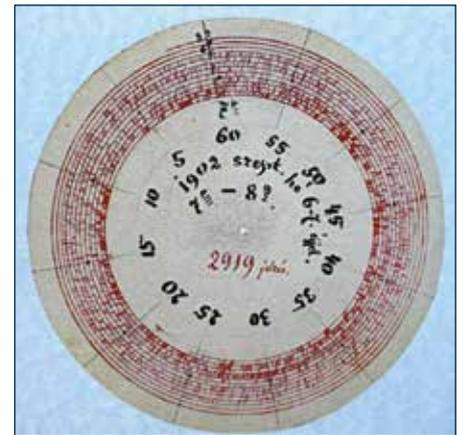
Fig. 16 One of the disk recorded in 1902 with Palatin's lightning recorder. (Tibor Horvát, 2001, op. cit. note 39).
