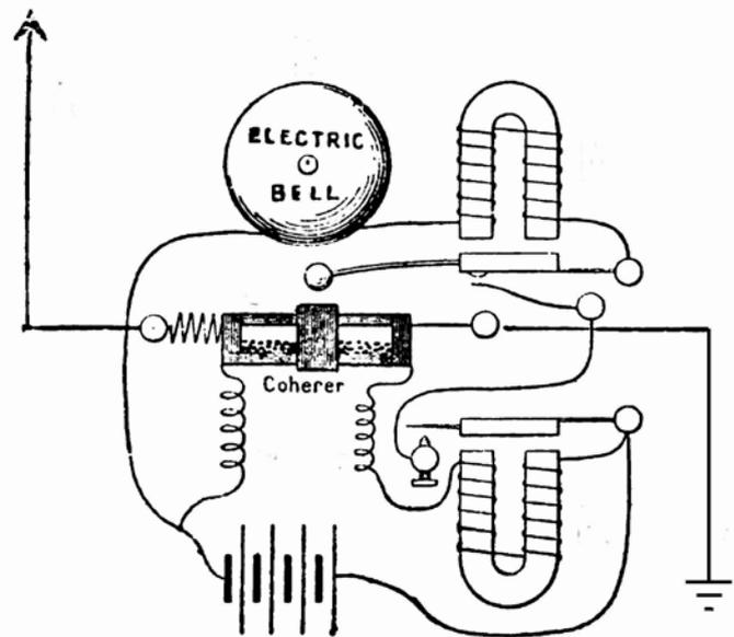
Fig. 10 *Original scheme of Popov's lightning detector. The same kind of circuit was used by several devices of the same type and by the early wireless receivers. (Popov, 1896, op. cit. note 30).*
