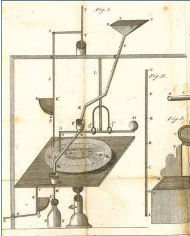
Fig. 3 Cavalli's cronio-ceraunometer. The cronimeter recorded the hour and then quantity of rain on the internal ring of the clockwork driven disk. The quadrangular funnel collected the rain which filled the small vessel fixed on the lever with a pen. Electric discharges were recorded with the ceraunograph on the external part of the disk. The bar connected to the lightning rod and the one going to the ground are equipped with quadrant electrometers. (Cavalli, 1785, op. cit. note 8).
