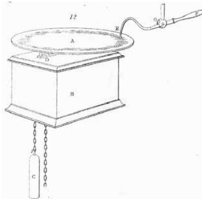
Fig. 8 The second simplified version of Ronalds electrograph. The resin covered disk was inserted on the arbour of the clockwork and rotated. The moveable arm was connected with a lightning rod. (Ronalds, 1845, op. cit. note 24).
