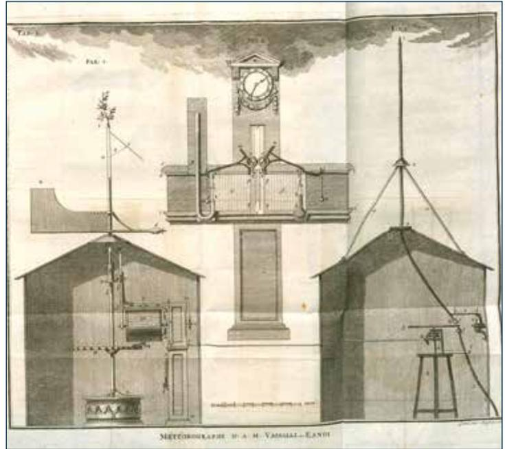
Fig. 4 The very complicated meteorograph proposed by Vassalli-Eandi. The recording anemometer and a recording wind vane with their recording drum are on the left; the barograph and the thermograph together with a clock are placed in the centre, while on the right there is the ceraunograph. The latter was actioned by a glass rod connected with the clockwork of the anemograph. (Vassalli-Eandi. 1803-4, op. cit. note 12).
