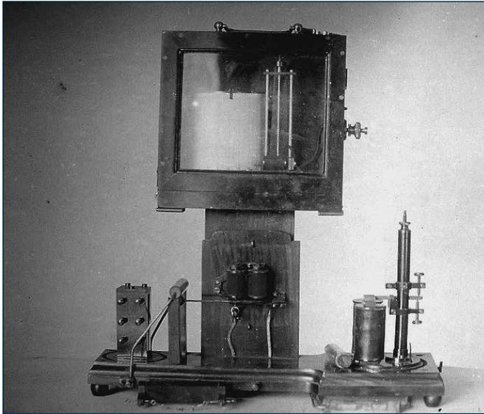
Fig. 17 An old photograph of the lightning recorder in use at the Gothard Observatorium. On the top of the instrument a Richard recorder. The instrument (without the recorder) is still preserved today. (See: <http://www.gothard.hu/gttak/archive-photos/categories/physmisc/physmisc.php>).
