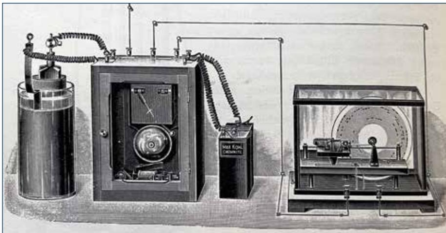
Fig. 15 The improved version of the Schreiber recording apparatus by the German manufacturer Max Kohl. On the left the detector, on the right the recording apparatus. (Max Kohl, 1905, op. cit. note 43).
