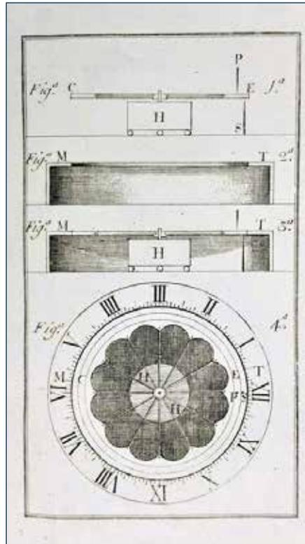
Fig. 1 The original ceraunograph described by Beccaria. The top image shows the disk inserted on the clockwork mechanism. P and S are the electrodes connected respectively with the lightning rod and with the ground. In the other images the instrument in its box with the horary dial. (Beccaria 1780, op. cit. note 2).
