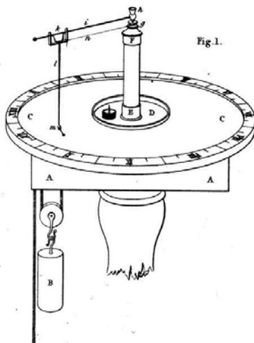
Fig. 7 The first Ronalds electrographs. The resin did not move, while the arm supporting the wire with the beads rotated on the resin disk. (Ronalds, 1823, op. cit. note 21).
