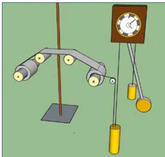
Fig. 2 A modern illustration reconstructing the second version of Beccaria's ceraunograph. The electric discharges were recorded on a long roll of paper passing between the two electrodes. The inscribed paper was rolled around a cylinder moved by the falling weight of a pendulum clock. (Diagram of the author).
