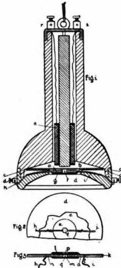
Fig. 13 This scheme illustrate Tommasina's electro-radiophone with the 'auto de-cohering coherer'. (Tommasina, 1901, op. cit. note 37).
