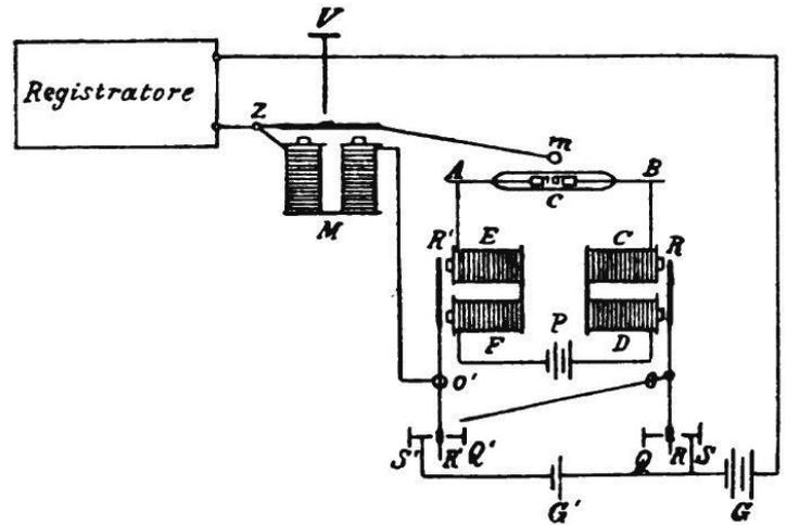
Fig. 12 This scheme illustrates the Boggio-Lera lightning recorder with two relays (R and R'). With it one could register in a different way the faint and far lightning and the stronger one of a local storm. (Boggio-Lera, 1900, op. cit. note 34).
