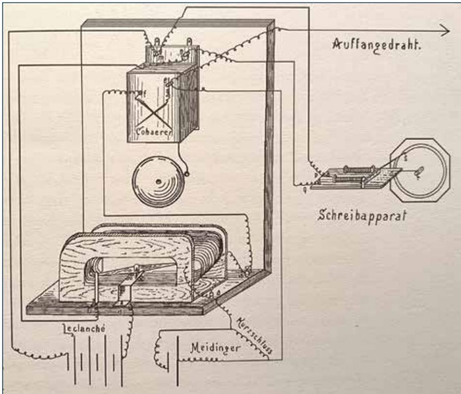
Fig. 14 Diagram illustrating the Schreiber and Fényi Gewitter-Registrator. The couple of crossed needles acting as cohaerer was on the box of the electric bell. The galvanometer was used instead of a telegraphic relay. (Tibor Horvát, 2001, op. cit. note 39).
